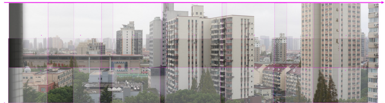
Fig. 15 Wide-field imaging based on vertical flight path LOS compensation 图15 基于垂直航迹视轴补偿的宽视场成像效果
