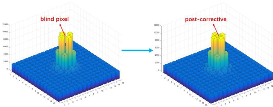
Fig. 13 Blind pixel point at the center of the spot
