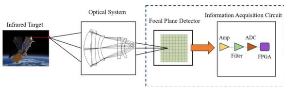
Fig. 1 Short-wave infrared imaging system
