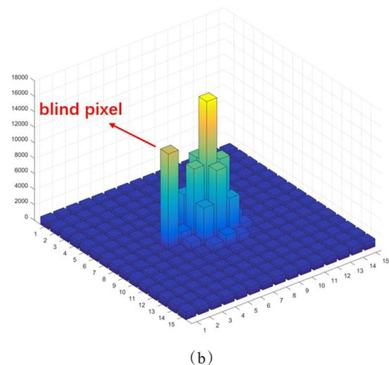
Fig. 2 Schematic diagram of a blind pixel with a Gaussian spot:
