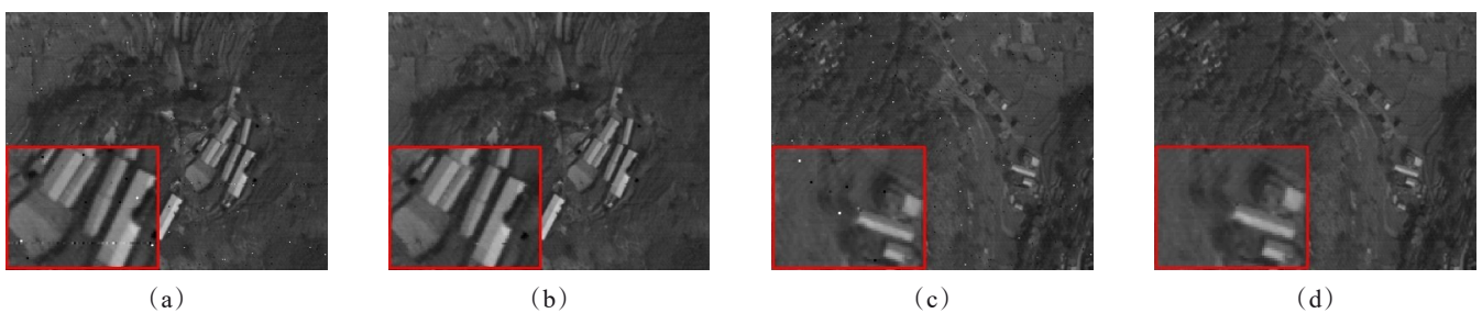
Fig. 11 (a) and (c) are the LWIR raw images; (b) and (d) are correspondingly noise-removed images 图11 (a)和(c)是长波红外原始图像; (b)和(d)是对应的噪声移除图像
