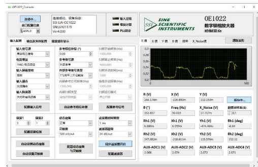
图18 锁相放大器显示的太赫兹探测响应波形 Fig. 18 Terahertz detection waveform displayed by a phase-locked amplifier
