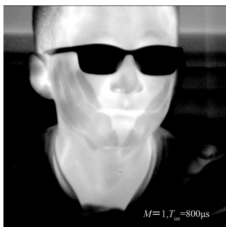
图 14 碲镉汞 APD 焦平面在 -50 mV 反偏下成像演示 Fig. 14 Imaging demonstration of a HgCdTe APD focal plane under V_{\text{bias}} = -50 mV
