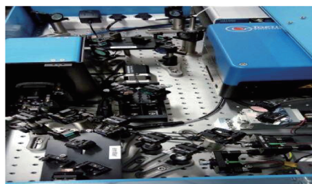
Fig. 9 Internal optical path map of transmission-type THz-TDS TDS 1008
