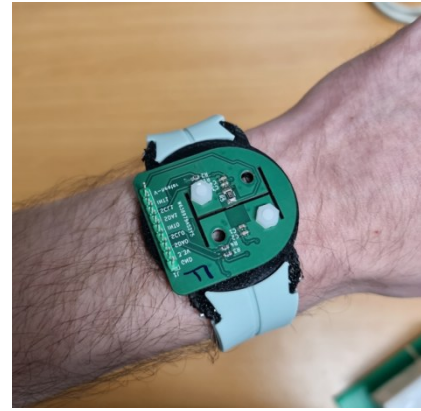
Fig. 6 The front side of the watch-like prototype for measuring wrist temperature
