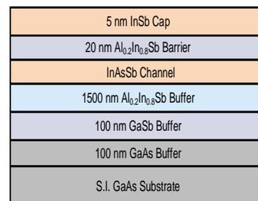
Fig. 2 Schematic diagram of  $\text{Al}_{0.2}\text{In}_{0.8}\text{Sb}/\text{InAs}_x\text{Sb}_{1-x}$  quantum well heterostructures
