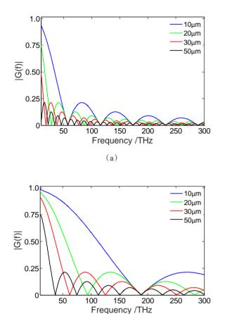
Fig. 2 The response function of the EOS with different GaSe thicknesses ( $10~\mu m$ ,  $20~\mu m$ ,  $30~\mu m$ , and  $50~\mu m$ ) with two different probe laser wavelengths: (a) is with 800 nm and (b) is with 1030 nm
