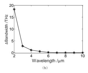
Fig. 5 The changing of (a) the central frequency and (b) the bandwidth depending on the wavelength of the few-cycle laser pulse from 2  $\mu$ m to 10  $\mu$ m
