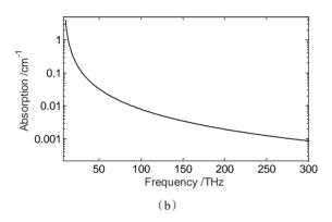
Fig. 1 (a) The ordinary and extraordinary light refractive indexes and (b) the absorption of GaSe crystal in the mid-infrared range 图 1 寻常光和非寻常光在硒化镓晶体中的(a)折射率和(b)吸收系数
