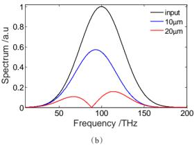
Fig. 4 The pulse distortions of few-cycle laser pulse with a wavelength of 3  $\mu m$  induced by the EOS with different thicknesses: (a) shows the time waveforms and (b) shows their frequency spectra
