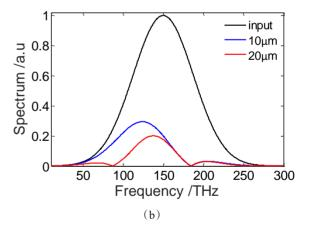
Fig. 3 The pulse distortions of few-cycle laser pulse with a wavelength of 2  $\mu m$  induced by the EOS with different thicknesses: (a) shows the time waveforms and (b) shows their frequency spectra, respectively
