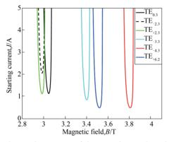
Fig. 3 The starting current of the operating mode and the main competitive mode varies with the external magnetic field, where the beam voltage of 30 kV, beam radius of 3.3 mm and transverse-to-axial velocity ratio of 1.3 were selected
