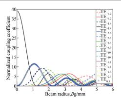
Fig. 2 The normalized beam-wave coupling coefficient of the dominant and competitive modes varies with beam radius 图 2 主模和竞争模式的归一化注波耦合系数随波束半径变化
