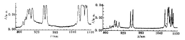
图 1 Nd3+: YAG 体材料的荧光光谱 Fig. 1 Fluorescent spectrum of Nd3+: YAG bulk material
