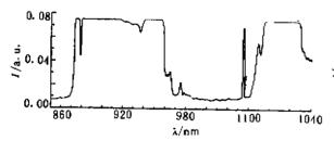
图 3 Nd<sup>1+</sup>: YAG 小球的荧光光谱 2 Fig. 3 Fluorescent spectrum 2 of Nd<sup>3+</sup>: YAG microsphere
