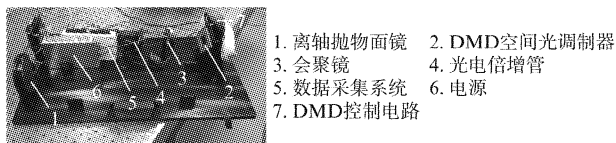
图 11 远距离对外成像实验装置实物图 Fig. 11 Photo of experimental device for long-range outdoor imaging experiments
